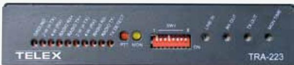
The TRA-223 tone-adapter is a simple way to remotely control radio base stations. The TRA-223 can be used in conjunction with all Telex analog consoles, or other manufacturers' consoles that use the industry-standard sequential tone keying format.
