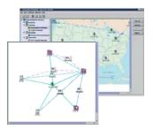
levels from regional network views down to the network element (NE). Logical topology shows visual representation of the links, interdependencies, and relationships among network devices. The physical topology provides visual representation of the actual device and any components residing inside. In addition, equipment locations can be managed according to region, cell or sector.
