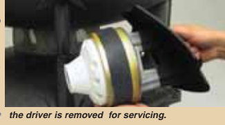
the driver is removed for servicing.
